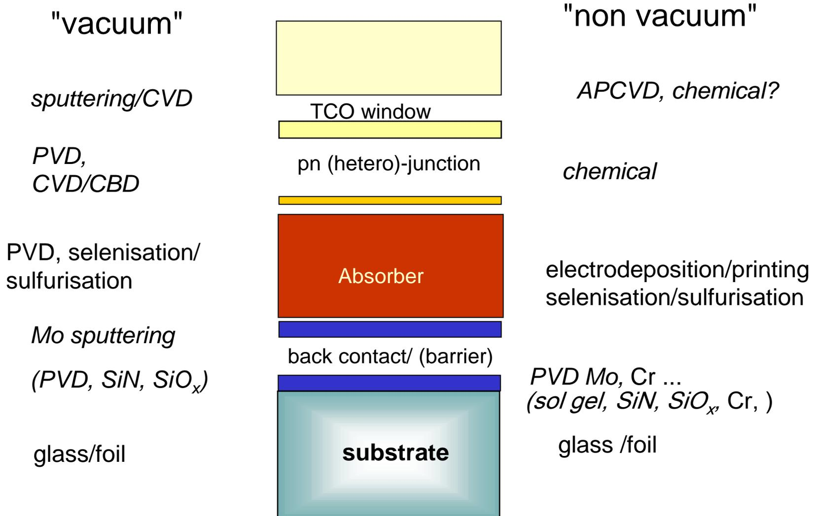
substrate structure enabling flexible cells by role-role manufacturing,
