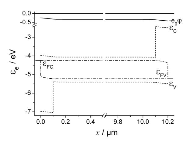
electrons and holes move against the field at max. power !!  $V_b = 697$  mV,  $V_{mpp} = 987$  mV
